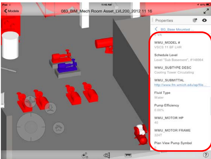
iPad screenshot navigating a BIM model, the properties box on the right shows the Mechanical Asset of the highlighted pump
