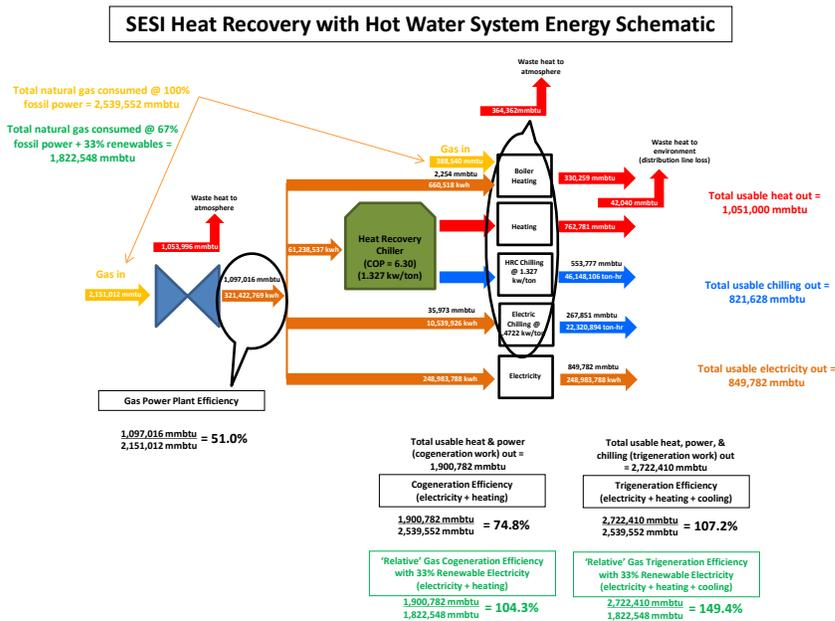
A similar energy schematic for the existing Cardinal Cogeneration plant serving Stanford shows that it consumes 52% more gas than the SESI plant will, assuming SESI electricity is derived from 100% fossil fuel. However, accounting for the 33% California RPS, the existing Cardinal Cogeneration plant consumes over twice the gas (3.8 mil mmbtu vs 1.8 mil mmbtu per year) required to meet campus energy needs under SESI.
