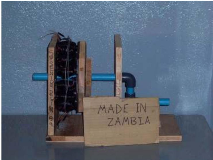
**Hand Cranked Generator capable of charging a cell phone – made entirely of locally available parts.**
