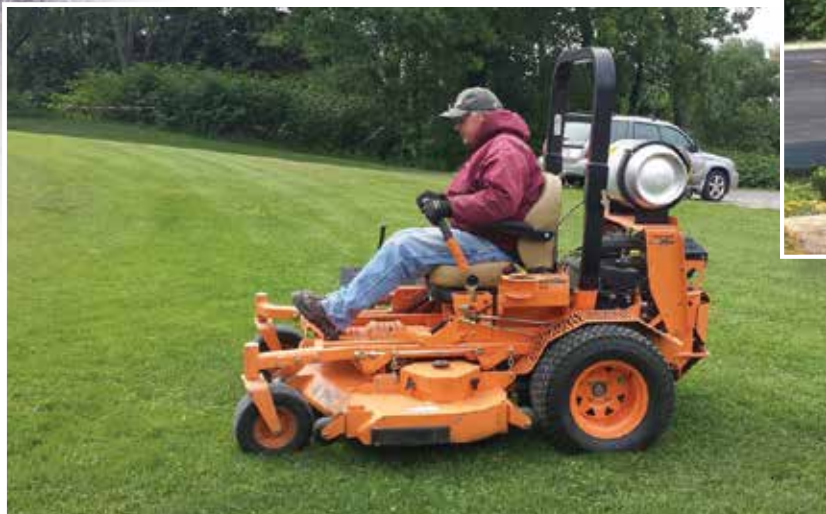
This propane powered ZTR mower requires less maintenance than the gas-powered ZTRs.
