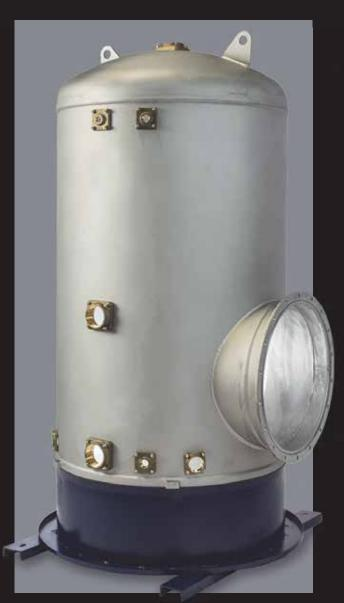
PVI fabricates AquaPLEX tanks and packages them into DOE-compliant and ETL-listed water heaters using natural gas, oil, electricity, boiler water or steam as the energy input. Dual-energy heaters are configurable for waste-heat capture, solar heating or off-peak energy usage. Storage tanks are available from 150 to 3000 gallons. Inputs range from 199,000 to several million BTU. All heaters are constructed and stamped to ASME code.
