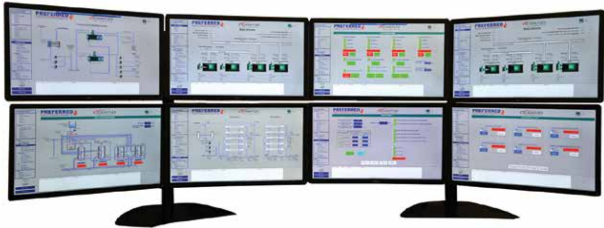
Remote monitoring system can be customized to full or more compact SCADA system (supervisory control and data acquisition).
