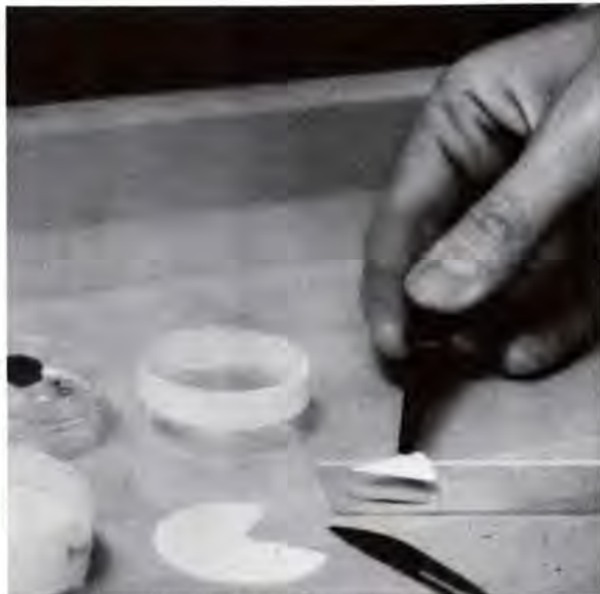
Mounting asbestos filters for phase contrast microscopy.
