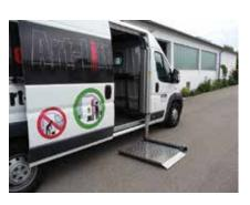
systems, the ArtLift is extremely lightweight, but it boasts a 440-lb. lifting capacity that accommodates more than 98 percent of common freight. A powerful 12-V electric motor provides the needed torque to smoothly rotate a
