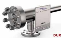
is simple in construction and consists of three fundamental components: a motive steam nozzle, suction body, and diffuser. The compact, lightweight design means it's easy to install into a pipeline, enabling overhead installations. A wide range of materials is available to suit process requirements to ensure maximum operating efficiency, including stainless steel, carbon steel, titanium, chrome, and molybdenum. For more information visit Spirax Sarco at *www.spiraxsarco.com/global/us*.
