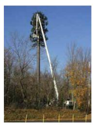
S-174 XDT allows you to drive to a location and raise the boom to precisely place the working platform almost anywhere on the tower. Setup is a breeze—a single control button activates the outriggers and leveling system, which can be positioned in less than a minute. Identical control panels are located on the platform and at the turntable control station for additional safety. For more information on Bronto Skylift visit *www.brontoskylift.com*. (§)
