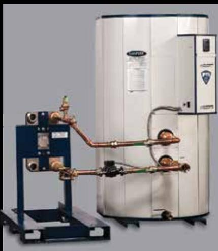
PVI's EZ Plate storage water heaters use a tank fabricated from AquaPLEX duplex stainless steel. The fully pickle-passivated tank is corrosion-proof in potable hot water regardless of temperature, needs no tank lining, needs no anode rods of any type and is backed by a 25-year corrosion warranty.\*
