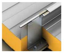
panels are available in 26-, 24-, and 22-gauge Galvalume/G90 galvanized and stainless steel. Exterior finish is standard gloss polyvinylidine fluoride coating. RidgeLine panels can be used on slopes as low as 1/2:12
