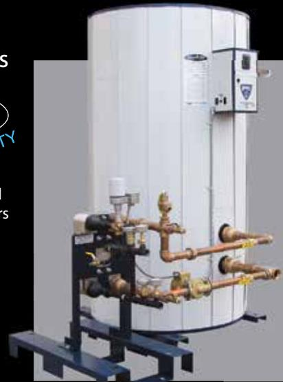
PVI's EZ Plate storage water heaters use a tank fabricated from AquaPLEX duplex stainless steel. The fully pickle-passivated tank is corrosion-proof in potable hot water regardless of temperature, needs no tank lining, needs no anode rods of any type and is backed by a 25-year corrosion warranty.
