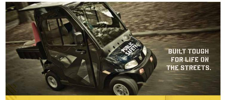
While the LSV 800 is street legal on most public roads with speed limits of 35 mph or less, this isn't just a joy ride. A 48-volt zero-emissions electric drivetrain, advanced hydraulic disc braking system and 5.9-cubic-foot cargo bed means this new crew member can hold its own on the job. **Visit Cushman.com/streetlegal to watch the LSV 800 in action and find an authorized Cushman® low speed vehicle dealer.**
