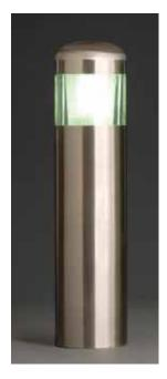
are constructed of an inner core of carbon steel to withstand high-speed impacts and an outer sleeve of Type 304 stainless steel for aesthetics and durability in harsh environments. For indepth information contact Calpipe Security Bollards at www. calpipebollards.com.
