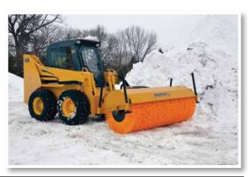
and come with a universal coupler for attaching to equipment with various hydraulic flow ratings. Additionally they can be hydraulically angled 30 degrees left or right. For in depth information please contact Pro-Tech at www.protechcorp.com.
