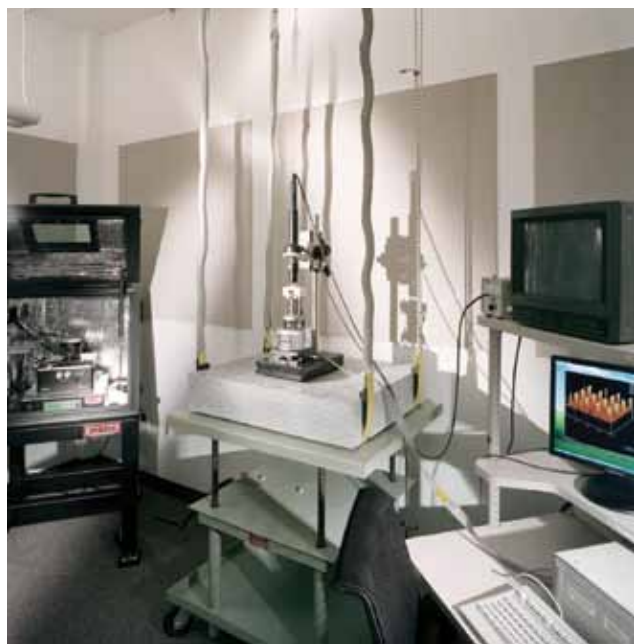
INERTIA BASE SUSPENDED WITH ELASTIC STRAPS
