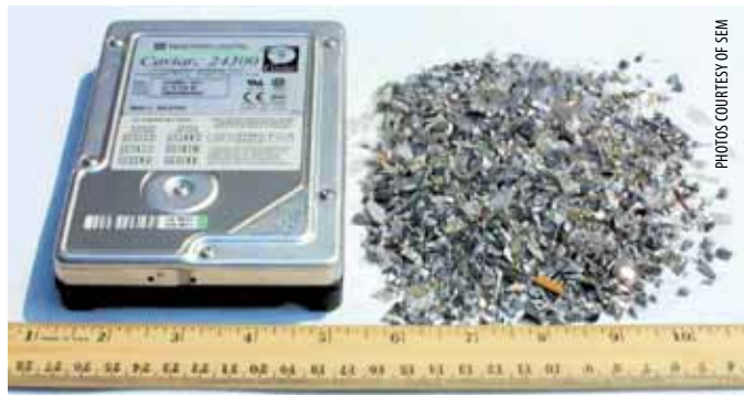
After passing through a disintegrator, computer hard drives end up as tiny bits of "e-scrap."
