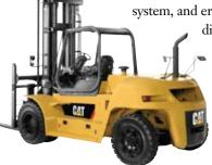
different capacities ranging from 17,500 to 36,000 lbs., these trucks are ready to tackle the most demanding customer applications. For optimal performance, the P17500 - P36000 relies on the turbocharged diesel
