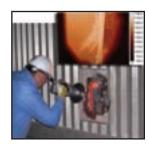
motors, bearings, etc. The camera offers three selectable temperature ranges, including a high-temperature (400°C - 1600°C) range needed for infrared imaging inside furnaces where combustion temperatures can exceed 1100°C. It also captures simultaneous visual images with on-board voice annotation. For additional details contact Mikron Infrared at 888-506-3900.
