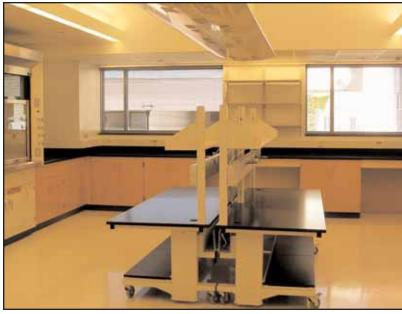
The research labs are open labs with no "anchor" type functions which would impede their flexibility. Overhead service carriers with all utilities greatly contribute to the flexibility.
