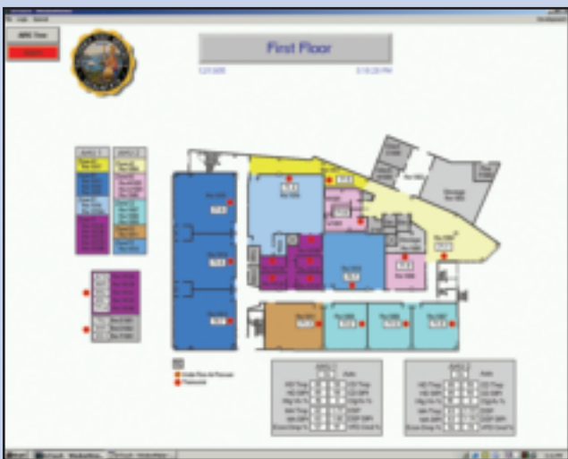
Typical floor plan with real time temperatures. Lower right corner provides real time information about the two air handlers serving the floor.
